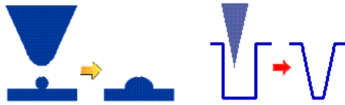
Figure 4: The final picture from the AFM is a convolution between the shape of the tip and the shape of the sample. [6]
